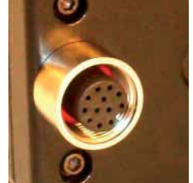
Closeup of optional isolated 24V I/O connector
