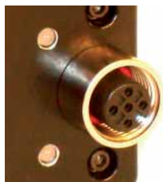
Closeup of optional CAN connector
