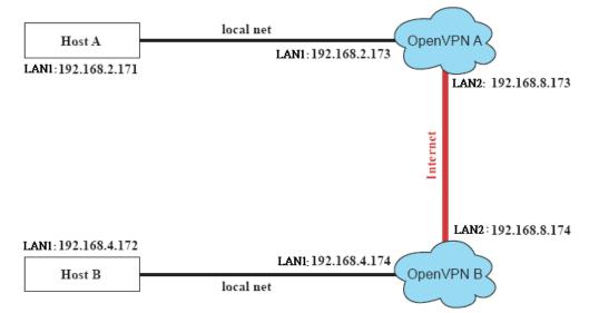
Host A represents the machine that belongs to OpenVPN A, and Host B represents the machine that belongs to OpenVPN B. The two remote subnets are configured for a different range of IP addresses. When this configuration is moved to a public network, the external interfaces of the OpenVPN machines should be configured for static IPs, or connected to another device (such as a firewall or DSL box) first.
