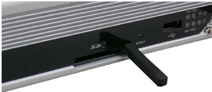
**Step 2:** After removing the cover, insert the SD memory card into the slot.
