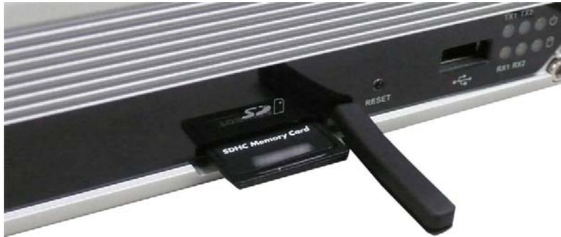
**Step 3:** Gently move the protective cover back to the SD slot. Power on the embedded computer and start the operating system.
