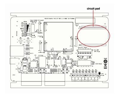
The bottom row of pins is for connecting a 5V power supply; the next row up is for connecting a 3.3V power supply. Digital I/O pins are located on the right side. The top row of pins is for grounding.
