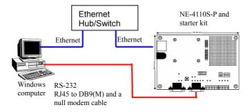
Note that for the serial-to-Ethernet version, P0 is the primary data port and P1 is used for the serial console port (3 wires). For the programmable version, **both P0 and P1 ports are freely programmable with the SDK**.
