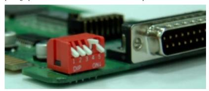
There are six base addresses from which to choose (see table below). Choose an address not being used by the expansion memory or other add-on cards. Note that if you want to add more than one C101/ISA board, each board must use a different IRQ number.
