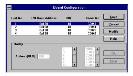
For example, if 4 ports are configured and starting from COM3, then the mapping of serial port numbers will be as depicted.
