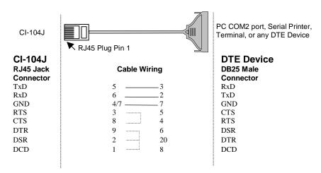
1 4/7 means either line 4 or line 7 can be used for GND.
