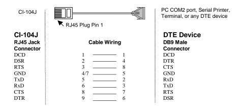
1 4/7 means either line 4 or line 7 can be used for GND.
