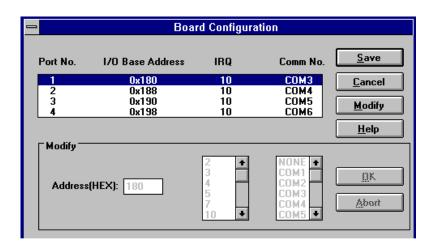
If you need to modify the settings, click [Modify], type in the desired I/O address in the "Address" field and select the desired IRQ and COM number. Then click [OK] and [Save] to save the new configuration and exit.
