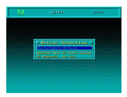
2. Press **Enter** to pop up the SETUP dialog box. In the SETUP dialog box, Press **F8** to specify the **CAP Address** and press **ENTER** and then type **Y** (**YES**) to load the configuration of the board to be setup.
