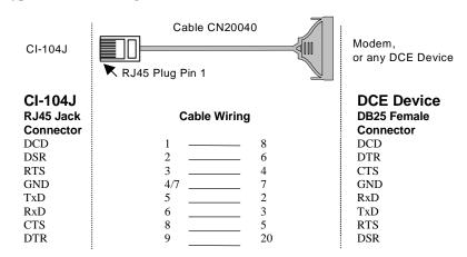
**Type 2:** Connecting Intellio CI-104J to a DCE device.
