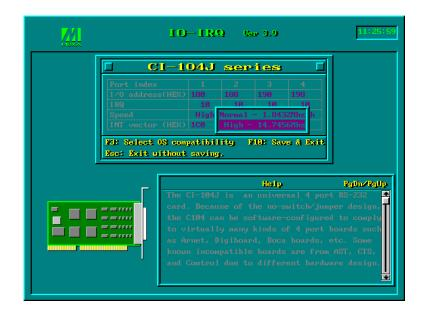
Note that, currently, port that uses MOXA Windows NT and 95/98 driver will run at the displayed speed. To be clear, when Smartio CI-104J Series board is configured as High Speed Spectrum, any port driven by the Moxa-provided Windows NT and 95/98 driver will display the exact working speed. For example, the displayed speed 38.4 Kbps is equal to the working speed 38.4 Kbps.
