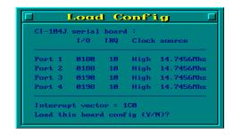
3. Now the configuration of the desired Smartio CI-104J Series board will be shown along with other default settings, such as port number, buffer size, etc.
