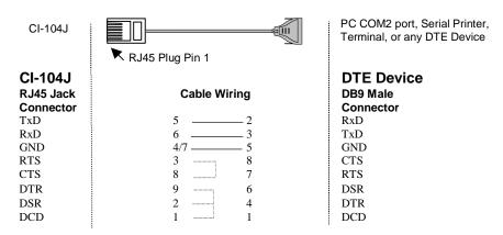
4/7 means either line 4 or line 7 can be used for GND.
