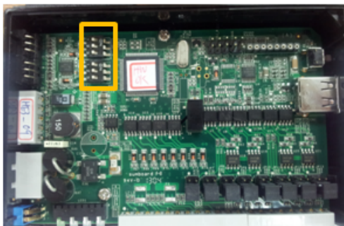
Pull High/Low DIP switch settings for the RS-485 Port
