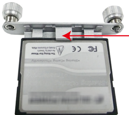
Put CF Card into tenon/hook of CF socket
