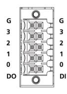
The UC-5100 Series comes with 4 digital inputs and 4 digital outputs. The DI/DO connectors are located on the top panel of the computer. Refer to the diagram on the left for the pin definitions. For the wiring method, refer to the following figure:
