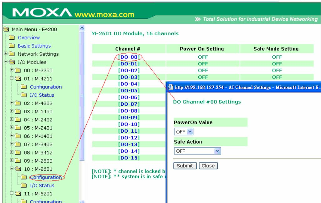
You may use the **PowerOn Value** field to specify the channel's setting when the ioLogik system is powered on, and the **Safe Status Setting** field to specify channel's setting when the ioLogik system enters Safe Status. Note that Safe Status is controlled by the Host Connection Watchdog, which is disabled by default. If the Host Connection Watchdog is disabled, the ioLogik system will never enter Safe Status and your Safe Status settings will have no effect.
