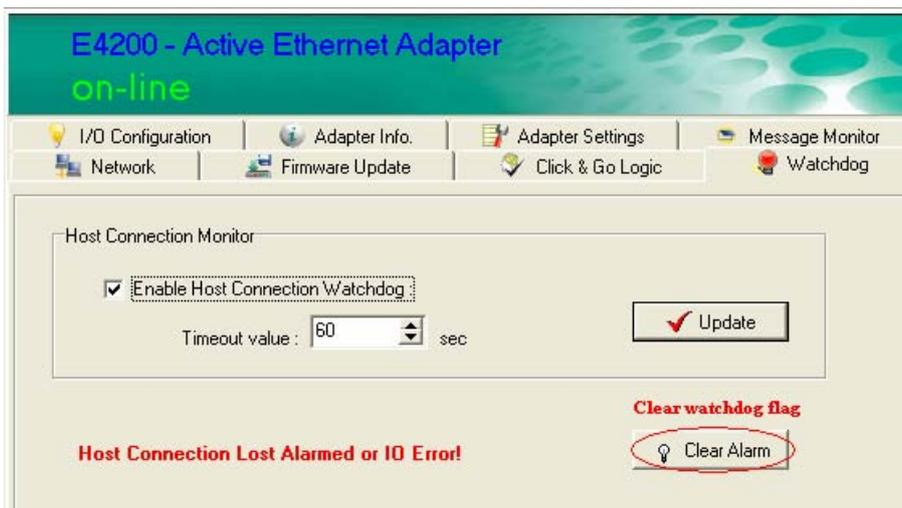
After the Watchdog is enabled, the ioLogik E4200 will enter safe status if the network connection is lost. Once the connection has been restored, you will need to return to the Watchdog Tab in order to exit safe status. There will be a message saying "Host Connection Lost", indicating that the I/O device is in safe status. Click **Clear Alarm** to exit safe status and return to normal operation.
