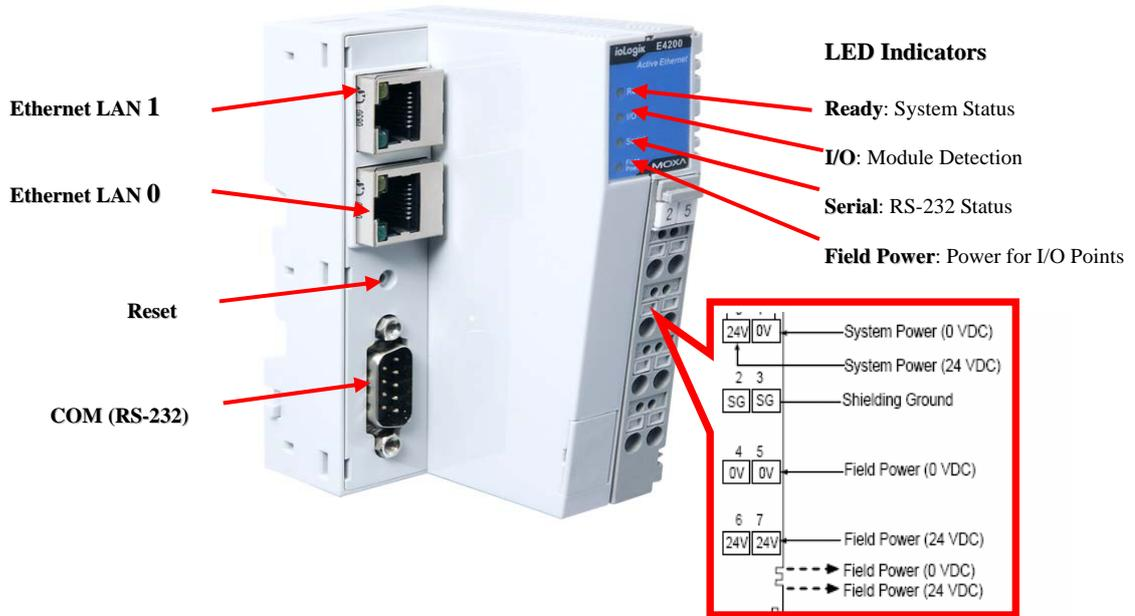
**NOTE:** The reset button restarts the system and resets all settings to factory defaults. Use a pointed object such as a straightened paper clip to hold the reset button down for 5 sec. The READY LED will turn red as you are holding the reset button down. The factory defaults will be loaded once the READY LED turns green again. You may then release the reset button.
