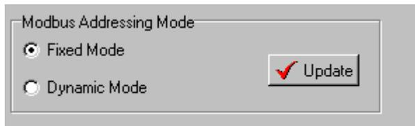
1. Fixed mode (Default): Every slot has its own memory bank. It is easy way to understand, but has lower efficiency due to large memory size.
