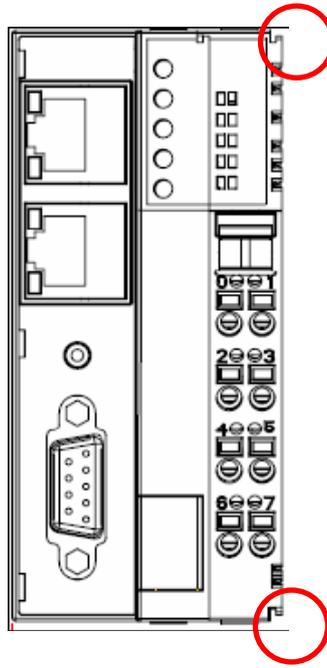
Step 2: Align the I/O module side by side with the network module and then push the I/O module until it touches the DIN-rail. Next, apply more force until the module clips to the DIN-rail.
