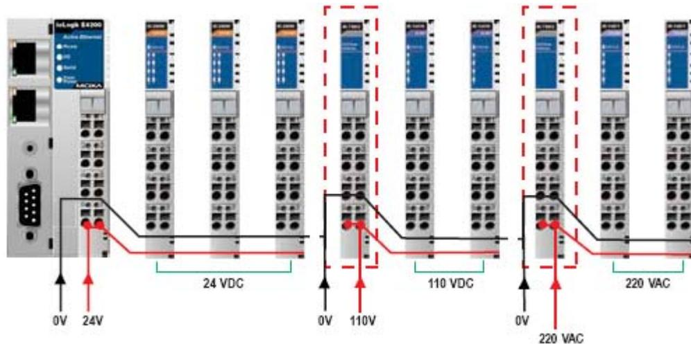
Some types of Potential Distributor modules provide extra wiring points such as shielding ground, field power 0V, and field power 24V. For example, the 8-channel digital input (sink type) module itself does not have a 24V wiring point. You may add a 24V Potential Distributor for easy wiring.
