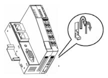
Step2: While still holding down the tab, pull out the Module.
