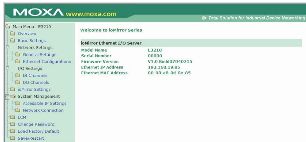
The main page of the web console displays detailed information about your ioMirror unit, including module name, serial number, firmware version, IP address, and MAC address.
