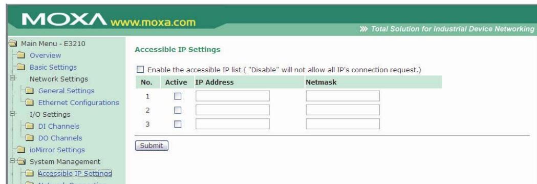
On the Accessible IP Settings page, you may control who has configuration access to the ioMirror by entering the permitted **IP Address** and **Netmask**. When the accessible IP list is enabled, only network hosts on the list may configure the ioMirror. Use the accessible IP list as follows:
