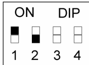
4-wire RS-422/485 without Termination Resistor
