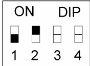
2-wire RS-485 with Termination Resistor
