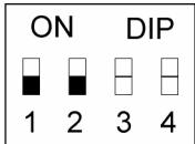
2-wire RS-485 without Termination Resistor
