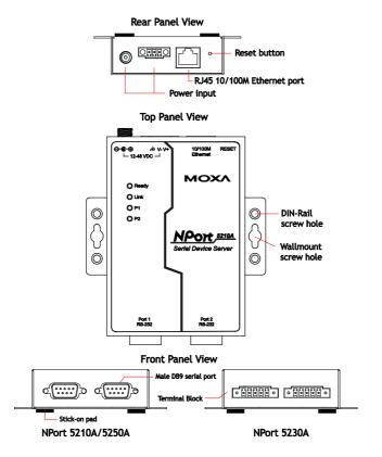
Reset Button—<u>Press and hold the Reset button for 5 seconds to load factory defaults</u>: Use a pointed object, such as a straightened paper clip or toothpick, to depress the reset button. This will cause the Ready LED to blink on and off. The factory defaults will be loaded once the Ready LED stops blinking (after about 5 seconds). At this point, release the reset button.
