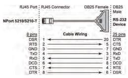
RJ45 (8-pin) to DB25 Male (Cable Name: CBL-RJ45M25-150)
