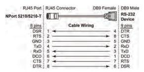
RJ45 (8-pin) to DB9 Male (Cable Name: CBL-RJ45M9-150)
