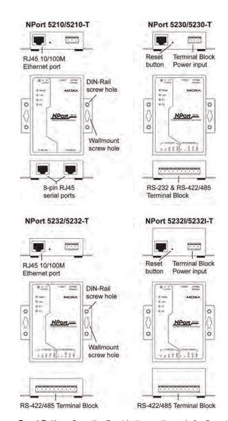
**Reset Button**—Press the *Reset button* continuously for 5 sec to load factory defaults: Use a pointed object, such as a straightened paper clip or toothpick, to press the reset button. This will cause the Ready LED to blink on and off. The factory defaults will be loaded once the Ready LED stops blinking (after about 5 seconds). At this point, you should release the reset button.
