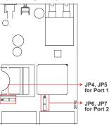
Jumpers are used to set the pull high/low resistors. The default is 150 K $\Omega$ . Short the jumpers to set this value to 1 K $\Omega$ . Do not use the K $\Omega$  setting with RS-232 mode, since doing so will degrade the RS-232 signals and shorten the communication distance.
