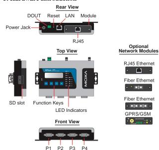
**Reset Button**—Press the Reset button continuously for 5 sec to load factory defaults: Use a pointed object, such as a straightened paper clip or toothpick, to press the reset button. This will cause the Ready LED to blink on and off. The factory defaults will be loaded once the Ready LED stops blinking (after about 5 seconds). At this point, you should release the reset button.
