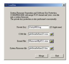
To generate a system firmware file, you will need to input the Private Key, original COM file, and Kernel file. The kernel file can be found in \SDK\FIRMWARE. After typing in the above information, type in a file name for the generated system firmware file. To download the system firmware, open SDK Manager and locate the target PCG. Select **Download System Firmware** under the Actions menu, or click on the **Download System Firmware** toolbar icon.
