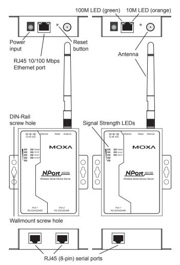
**Reset Button**—<u>Press the Reset button continuously for 5 sec to load</u> <u>factory defaults</u>: Use a pointed object, such as a straightened paper clip or toothpick, to press the reset button. This will cause the Ready LED to blink on and off. The factory defaults will be loaded once the Ready LED stops blinking (after about 5 seconds). At this point, you should release the reset button.
