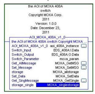
For "Switch\_Input" and "Switch\_Output", use the scrollbar to select the tag name
