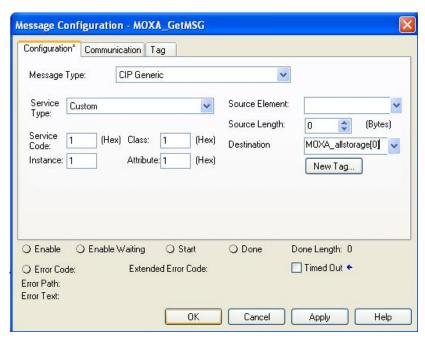
Click the **Communication** tab and set up the communication path to the Moxa Ethernet switch for **Get\_AllMessage**
