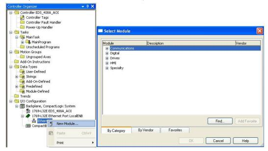
3. Under the **Communications** group, select **Generic Ethernet Module** to represent Moxa Ethernet switches
