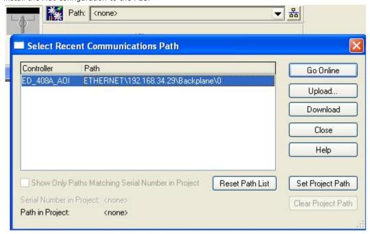
After finishing configuration, go to the controller organizer window, right click Controller Tags and select Monitor Tags to check if each tag can display the correct value transferred from the Ethernet device.
