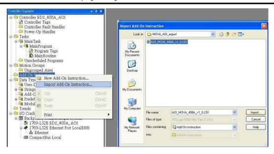
2. After importing, the controller organizer window shows all AOI for Moxa Ethernet switches under the **Add-On Instructions** folder.
