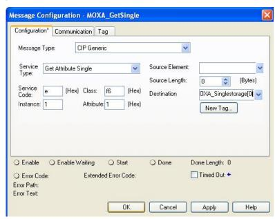
Click the **Communication** tab and set up the communication path to the Moxa Ethernet switch for **Get\_SingMessage**
