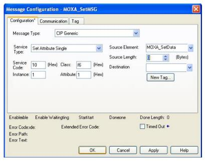
Click the **Communication** tab and set up the communication path to the Moxa Ethernet switch for **Set\_Message**
