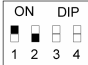
4-wire RS-422/485 without Termination Resistor
