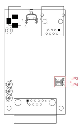
To set a pull high/low resistor to 150  $K\Omega$ , make sure that the two jumpers (JP3 and JP4) assigned to the serial port are not shorted by jumper caps. This is the default setting.
