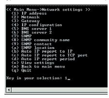
6. Use the Backspace key to erase the current IP address, type in the new IP address, and then press Enter.
