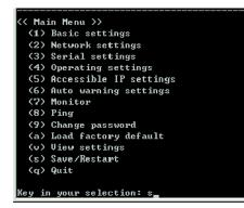
10. Type y and then press Enter to save the new IP address and restart the NPort 5100.
