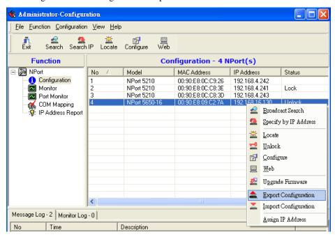
The Import Configuration function is used to import an NPort configuration from a file into one or more of the same model NPort.
