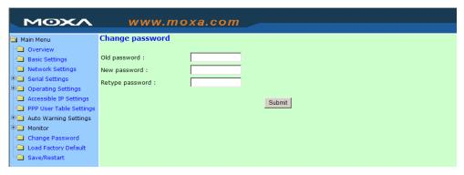
Input the "Old password" and "New password" to change the password. Leave the password boxes blank to erase the password. In this case, the NPort will not have password protection.
