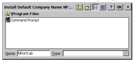
3. Driver installation is now complete and the "NPortCab.cab" icon disappear from the screen. This is normal when installing drivers in Windows CE.
