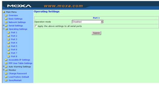
When Operation mode is set to Disabled, that particular port will be disabled. Select the *Apply the above settings to all serial ports* option to apply this setting to the other ports.
