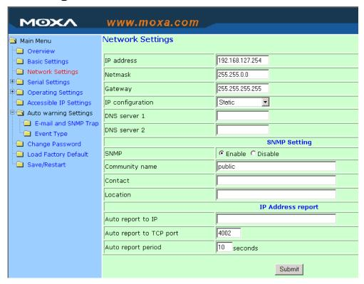
You must assign a valid IP address to NPort 5600 before it will work in your network environment. Your network system administrator should provide you with an IP address and related settings for your network. The IP address must be unique within the network (otherwise, NPort 5600 will not have a valid connection to the network). First time users can refer to Chapter 3, *Initial IP Address Configuration*, for more information.
