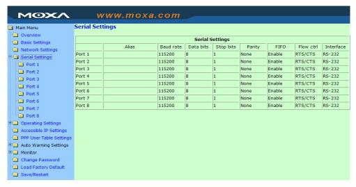
To modify serial settings for a particular port, click either **Port 1** or **Port 2** under **Serial Settings**, located under **Main Menu** on the left side of the browser window
