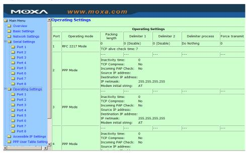
Click **Operating Settings** located under **Main Menu**, to display the operating settings for all of NPort's serial ports.
