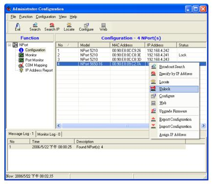
3. After entering the correct password, the Administrator will display a message box as shown here. The NPort is now unlocked.
