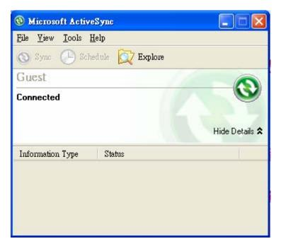
Step 3: Click on the "Explore" button in the ActiveSync window, and then copy the UP1100\_COM\_v1.0\_Setup.CAB (For WinCE 6.0) or UP1100\_COM\_v1.1\_Setup.CAB (For WinCE 5.0) file to the Mobile/Target Device.
