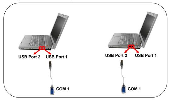
When "Fixed-base COM Mode" is enabled for the first time, all the COM port numbers and serial port parameters will reset to their default values. You can then set the COM numbers and configuration parameters to the values needed for your application(s). Note: If you subsequently disable "Fixed-base COM Mode," all the parameters will be restored to their original settings.
