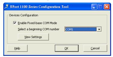
The COM numbers are assigned sequentially, and are not tied to a specific UPort device or USB port number. For example, let's assume that you've set COM1 as the first COM number that will be assigned. If a UPort 1150 is plugged into your computer's USB port 1, your computer assigns COM1 to the UPort's serial port. When the UPort 1150 is plugged into USB port 2, the computer still assigns COM1 to the UPort's serial port.
