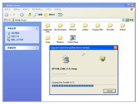
**Step 4:** Double click on the CAB file to start installing the UPort 1100 series WinCE driver. After installing the driver, plug the UPort 1100 series device into the USB port of the WinCE Device. The driver will be loaded automatically. At this point, the UPort 1100 series is ready to use.
