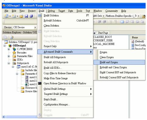
**Step 8:** After building sysgen, select "**Build**" and "**Make Run-Time Image**" to create the WinCE OS image. Finally, copy your image file to the target Host.
