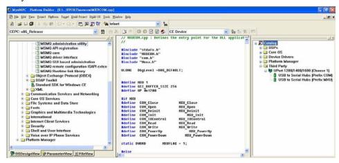
Step 3: Right-click on the driver "USB to Serial Adaptors (Prefix COM)" or "USB to Serial Adaptors (Prefix MXU)" and then choose "Add to OS Design." After adding the driver, you should be able to find it in your workspace. At this point, you can start building your operating system and download it to a target.
