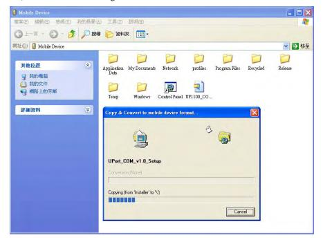
Step 4: Double click on the CAB file (UPort\_COM\_v1.0\_Setup.cab (Win CE 6.0) or UPort\_COM\_v1.1\_Setup.cab (Win CE 5.0)) to start installing the UPort 1200/1400/1600 Series WinCE driver. After installing the driver, plug the UPort 1200/1400/1600 Series USB Serial device into the WinCE device's USB port. The driver will be loaded automatically, after which the UPort 1200/1400/1600 will be ready to use.
