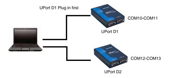
If both UPorts are unplugged from the computer, and then UPort D2 is plugged back in, the computer will now assign COM10 and COM11 to the UPort's serial ports. When UPort D1 is plugged back in, COM numbers COM12 and COM13 will be assigned the UPort's serial ports.
