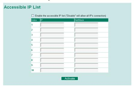
Accessible IP Settings allows you to add or remove *Legal* remote host IP addresses to prevent unauthorized access. Access to the EDS is controlled by IP addresses. That is, if a host's IP address is in the accessible IP table, then the host will be allowed access to the EDS. You can allow one of the following cases by setting this parameter
