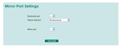
The **Mirror port** function can be used to monitor data being transmitted through a specific port. This is done by setting up another port (the *mirror port*) to receive the same data being transmitted from, or both to and from, the port under observation. This allows the network administrator to "sniff" the observed port and thus keep tabs on network activity.
