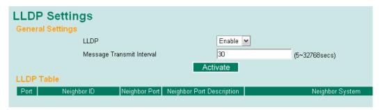
From the switch's web interface, users have the option of either enabling or disabling the LLDP, as well as setting the LLDP transmit interval (as shown in the figure below). In addition, users are able to view each switch's neighbor-list, which is reported by its network neighbors. Most importantly, enabling the LLDP function allows Moxa's MXview to automatically display the network's topology as well as system setup details such as VLAN, and Trunking for the entire network.
