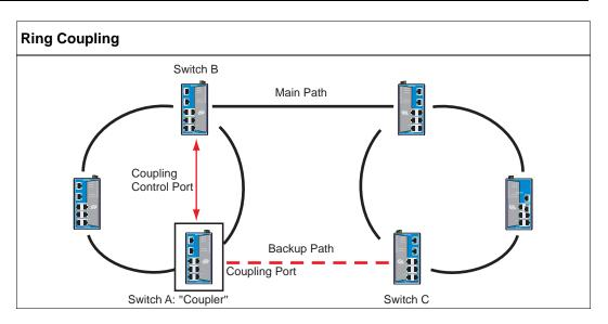
To support the Ring Coupling function, select one EDS (e.g., Switch A in the above figure) in the Turbo Ring and enter the Communication Redundancy page to enable "Ring Coupling." Select one port as "coupling port" and then connect any port of the opposing EDS (e.g., Switch C) in the adjacent Turbo Ring. Select another port as "coupling control port," and connect this port to any port of the adjacent EDS (e.g., Switch B) in the same Turbo Ring.
