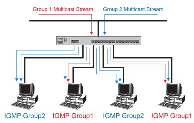
All hosts receive the multicast traffic, even if they don't need it. Network with multicast filtering
