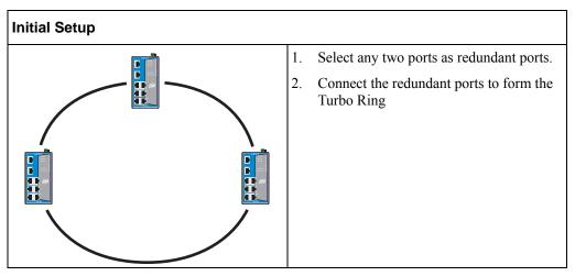
The user does not need to set the master to use Turbo Ring. Master is only needed to identify which segment acts as the backup path. The actual topology of the redundant ring, i.e., which segment will be blocked, is determined by the number of EDSs that make up the ring and where the "Ring Master" is located.
