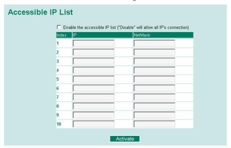
Accessible IP Settings allows you to add or remove "Legal" remote host IP addresses to prevent unauthorized access. Access to the EDS-516A is controlled by IP address. If a host's IP address is in the accessible IP table, then the host will be allowed access to the EDS-516A. You can allow one of the following cases by setting this parameter:
