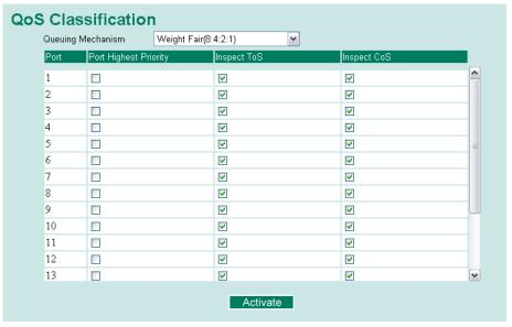
The EDS-516A supports inspection of layer 3 TOS and/or layer 2 CoS tag information to determine how to classify traffic packets.
