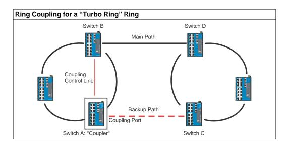
To configure the Ring Coupling function for a "Turbo Ring" ring, select two EDS-516A units (e.g., Switch A and B in the above figure) in the ring, and another two EDS-516A units in the adjacent ring (e.g., Switch C and D).
