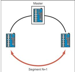
If there are 2N+1 EDS-516A units (an odd number) in the "Turbo Ring" ring, with EDS-516A units and segments labeled counterclockwise, then segment N+1 will serve as the backup path.
