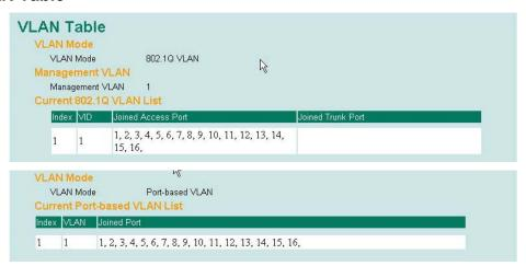
In 802.1Q VLAN table, you can review the VLAN groups that were created, Joined Access Ports, and Trunk Ports, and in Port-based VLAN table, you can review the VLAN group and Joined port.
