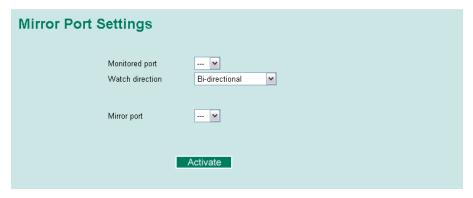
The **Mirror port** function can be used to monitor data being transmitted through a specific port. This is done by setting up another port (the *mirror port*) to receive the same data being transmitted from, or both to and from, the port under observation. This allows the network administrator to "sniff" the observed port and thus keep tabs on network activity.
