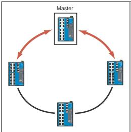
For a "Turbo Ring V2" ring, the backup segment is the segment connected to the 2nd redundant port on the master.
