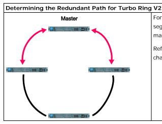
For **Turbo Ring V2**, the backup segment is the segment connected to the 2nd redundant port on the master.
