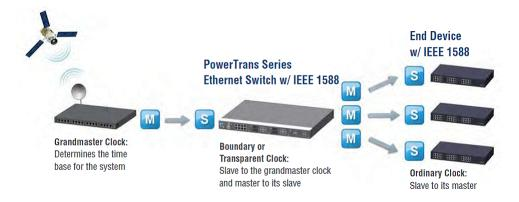
The following diagram shows a basic IEEE 1588 application hierarchy for substation automation.
