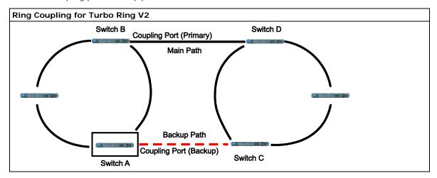
Note that the ring coupling settings for a **Turbo Ring V2** are different from a **Turbo Ring**. For Turbo Ring V2, ring coupling is enabled by configuring the **Coupling Port (Primary)** on Switch B and the **Coupling Port (Backup)** on Switch A only. You do not need to set up a coupling control port, so **Turbo Ring V2** does not require a coupling control line.
