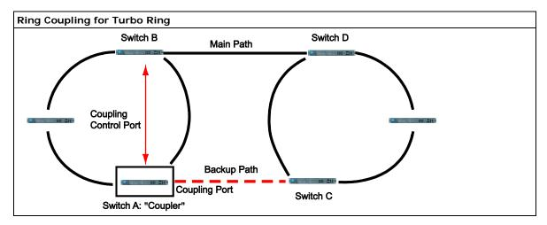
To configure the ring coupling for a **Turbo Ring**, select two PT series Ethernet switches (e.g., Switch A and Switch B in the above figure) in the ring, and another two PT series Ethernet switches in the adjacent ring (e.g., Switch C and Switch D).
