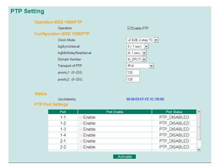
Configuration IEEE 1588/PTP of v2 E2E 2-step TC, v2 E2E 1-step TC and v2 P2P 2-step TC mode
