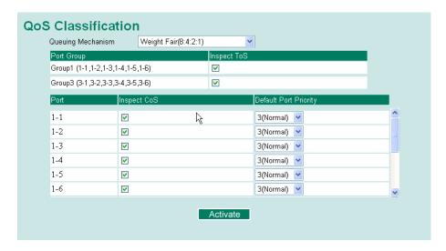
The PT-7728-PTP supports inspection of layer 3 TOS and/or layer 2 CoS tag information to determine how to classify traffic packets.
