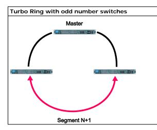
If the number of Ethernet switches in the Turbo Ring is 2N+1 (an odd number), the backup segment is the (N+1)st segment counting counterclockwise.
