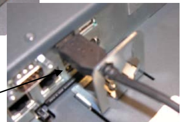
ePC-Series USB Retention Bracket
