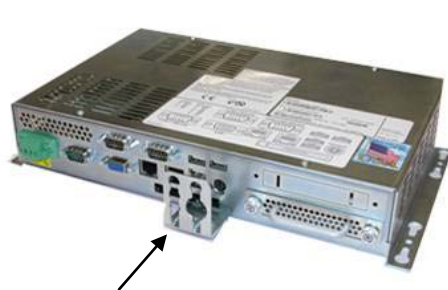
nPC100 USB Retention Bracket
