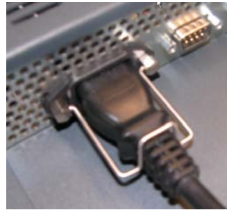
Power Cable Retention Clip Installed
