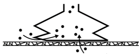
Figure 3.5: Visualization of leakage possibilities.
