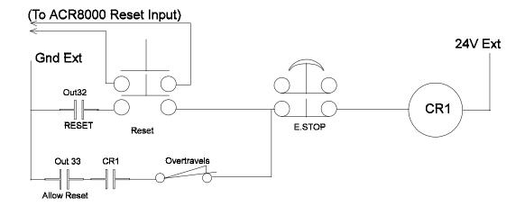
Note that the above circuit is 24 Volt DC ladder logic.
