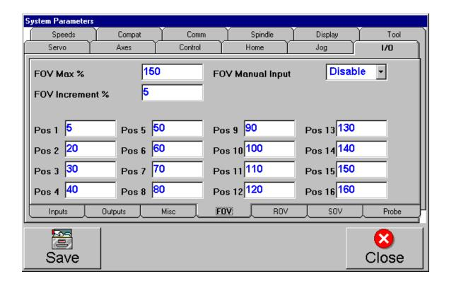
The "**Maximum**" override percentage is usually set to 100% and is meant to avoid the operator turning the FOV too high.
