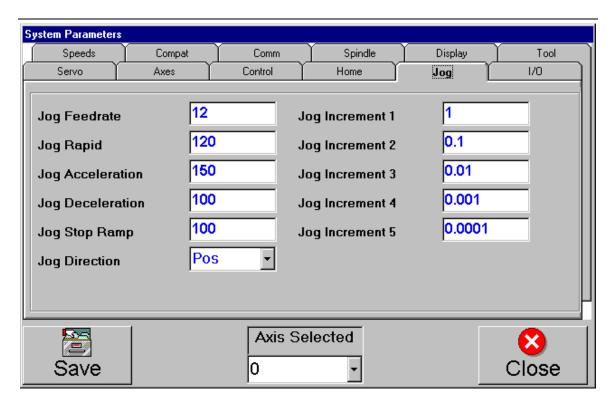
This screen allows different ACC/DEC and increments for each axes to be programmed.
