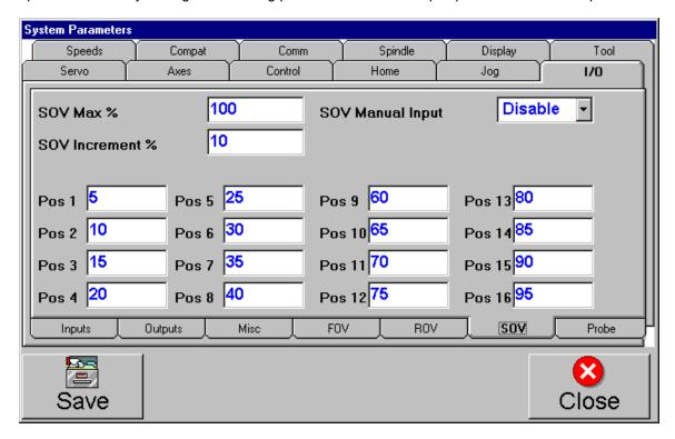
The "Maximum" override percentage is usually set to 100% and is meant to avoid the operator turning the SOV too high.
