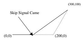
At the instant that the Skip Signal comes, the encoder positions are stored in parameters #201,#202,#203,#204,#205,#206,#207,#208 for axis X,Y,Z.....
