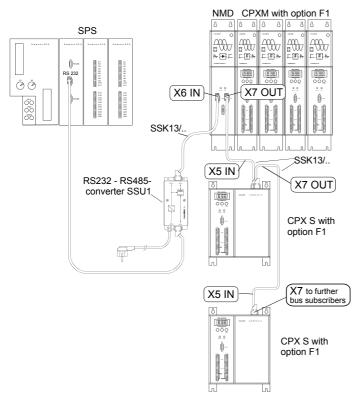
In a system group comprising a number of COMPAX devices and a power module (NMD), the RS485 signals are transferred over the already existing ribbon-cable connections.
