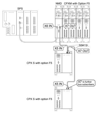
Within a system group of COMPAX M and a power module, the CAN-bus-signals are transmitted via the already existing ribbon cable connection.
