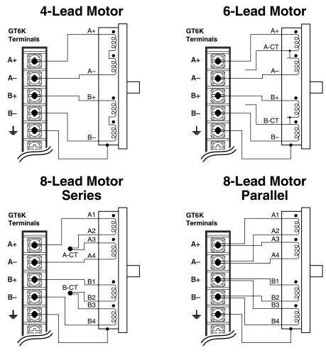
Non-Compumotor Motor Connections
