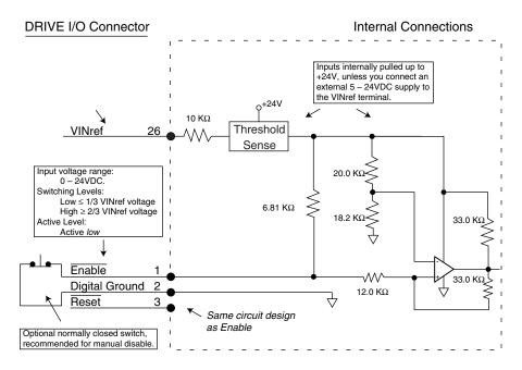
Enable Input and Reset Input
