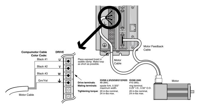
Motor Wiring with GV6K - Typical
