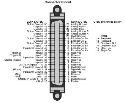
This section describes all inputs and outputs (I/O) located on the 50 pin DRIVE I/O connector. The connector pinout is shown in the next drawing.
