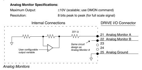
You can configure the analog outputs to monitor many different variables, such as current, velocity, temperature, etc. You can also scale the outputs. See the DMON commands in *Chapter 3 Configuration* and the *Gemini GV6K/GT6K Command Reference* for more information.
