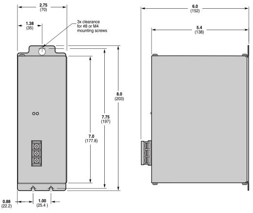
Dimensions – GPDM Power Dissipation Module
