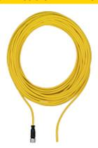
Connecting cable with plug, M12-12pin connector, female, 10m PUR-cable,  $12x0,25mm^2$
