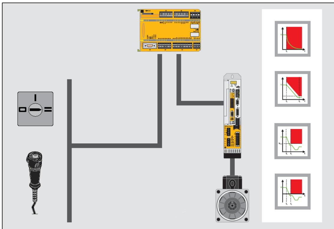
The example shows the implementation of the "Setting – Safely limited speed when an enable switch is operated" mode with an operating mode selector switch, an enable switch, a PNOZmulti and a PMCprotego D in combination with a PMCprotego S2 safety card.
