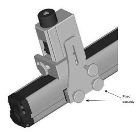
Now screw bracket [3] to bracket [1] using the fourth threaded knob. Now you can tighten up the two threaded knobs that connect [3] to [2].
