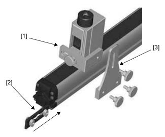
Push the holder [2] from above into the lateral groove until the required position is reached. Ensure that the retaining cams are vertical to the holder's longitudinal axis.
