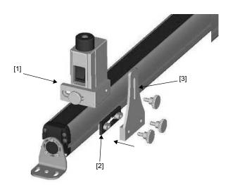
Insert the holder [2] into the groove, directly at the required position. Ensure that the retaining cams are parallel to the holder's longitudinal axis. Rotate the cams into the vertical position as soon as they are inserted in the groove.
