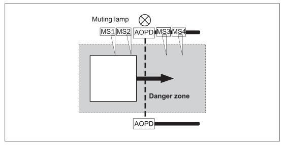
Muting sensors MS1 and MS2 must energise within 3 s (simultaneity). Muting starts when both muting sensors are active. The inputs of light guards S11-S12, S21-S22 and S31-S32 are muted. Status indicators "S1+S2" (Muting active), "S1", "S2" "OSSD CH.1" and "OSSD CH.2" are lit. A high signal is present at semiconductor output Y32 (muting active).
