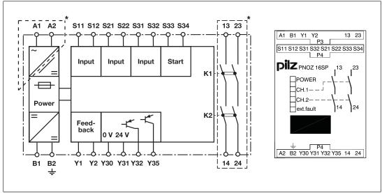
\*Insulation between the non-marked area and the relay contacts: Basic insulation (over-voltage category III), Protective separation (overvoltage category II)
