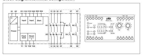
\*Insulation between the non-marked area and the relay contacts: Basic insulation (overvoltage category III), Protective separation (overvoltage category II)
