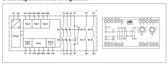
\*Insulation between the non-marked area and the relay contacts: Basic insulation (over-voltage category III), Protective separation (overvoltage category II)
