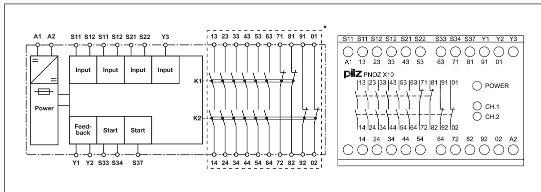
\*Insulation between the non-marked area and the relay contacts: Basic insulation (over-voltage category III), Protective separation (overvoltage category II)
