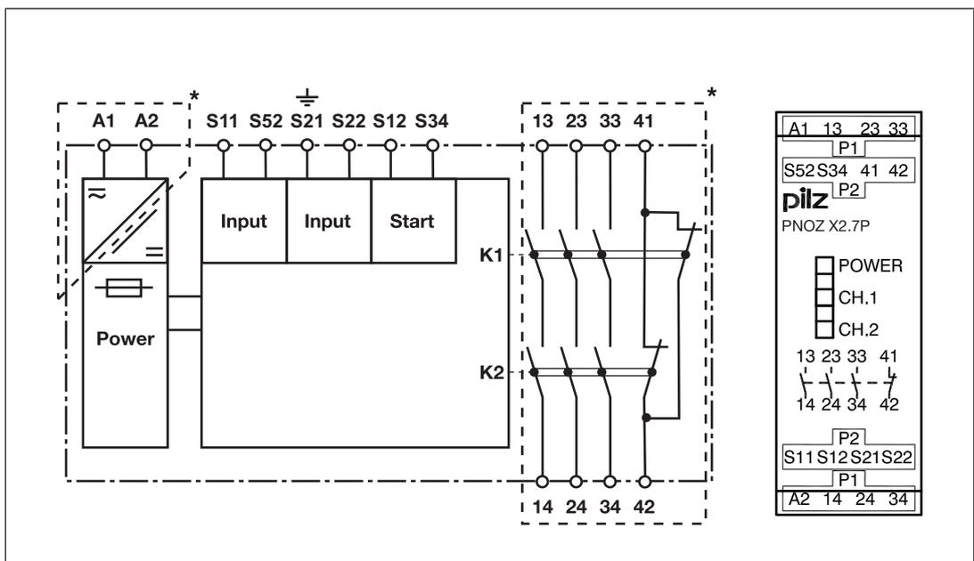
\*Insulation between the non-marked area and the relay contacts: Basic insulation (over-voltage category III), Protective separation (over-voltage category II)
