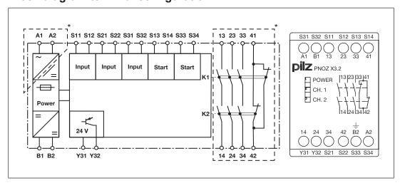
\*Insulation between the non-marked area and the relay contacts: Basic insulation (over-voltage category III), Protective separation (overvoltage category II)
