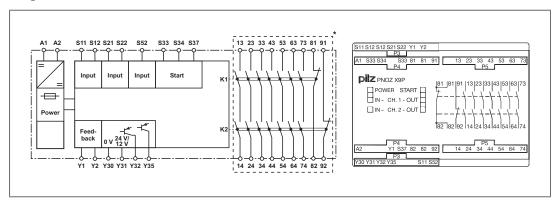
\*Insulation between the non-marked area and the relay contacts: Basic insulation (over-voltage category III), Protective separation (overvoltage category II)
