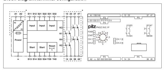
\*Insulation between the non-marked area and the relay contacts: Basic insulation (over-voltage category III), Protective separation (overvoltage category II)
