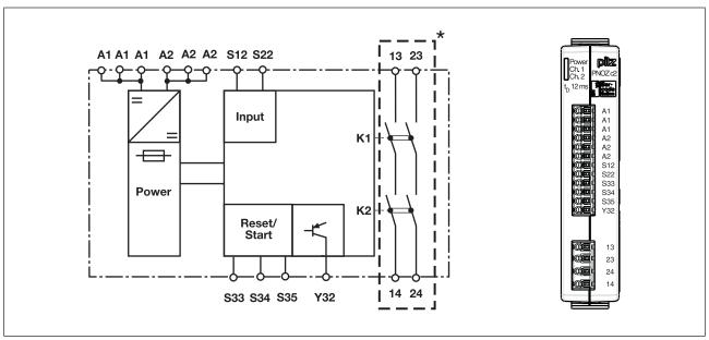
\*Insulation to the non-marked area: Protective separation (overvoltage category III), Insulation of relay contacts against each other: Basic insulation (overvoltage category III), protective separation (overvoltage category II)
